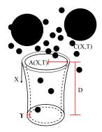
Figure 3: Schematic showing the single unit of membrane with a thin shell. Small particles, at concentration C(X,T), which enter pores and deposit within, are indicated, as are large particles, which block the pore inlet.
