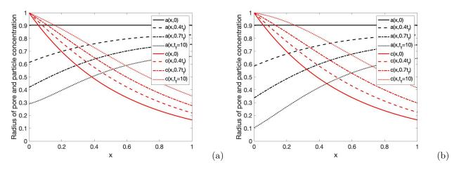
Figure 4: (a) is the pore radius and particle concentration at selected times up to 10 under thick wall model, as indicated in the legends; (b) is the pore radius and particle concentration at selected times up to 10 under thin wall model, as indicated in the legends. Both simulations are for uniform initial pore radius profiles a(x, 0) = 0.904.
