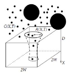
Figure 2: Schematic showing the single unit of membrane, assumed repeated in a square lattice. Small particles, at concentration C(X,T), which enter pores and deposit within, are indicated, as are large particles, which block the pore inlet.
