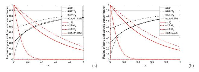
Figure 6: (a) is the pore radius and particle concentration at selected times up to the final blocking time ( $t_{\rm f} = 11.025$ ) under thick wall model, as indicated in the legends; (b) is the pore radius and particle concentration at selected times up to the final blocking time ( $t_{\rm f} = 9.975$ ) under thin wall model, as indicated in the legends. Both simulations are for uniform initial pore radius profiles a(x, 0) = 0.904
