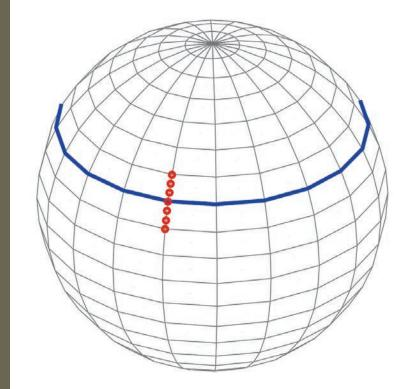
The newly developed quasi-backscattering set-up uses a line of receivers extending a small distance in one dimension from a transmitter.
