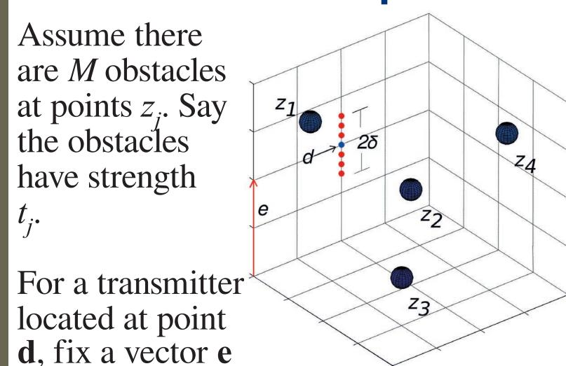
which is orthogonal to d. Place receiving devices at the locations  $\mathbf{x} = -\mathbf{d} + \eta \mathbf{e}$  where  $\eta$ ranges between the small parameter  $-\delta$  and  $\delta$ . The incident field has wave number k.
