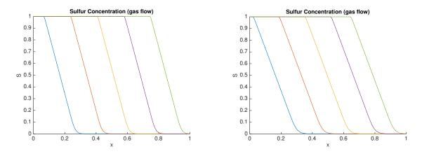
Figure 1: Behavior of S(x,t) for five intervals of time from t = 0 to  $t = t_{\text{final}}$ . Left: field simulation,  $t_{\text{final}} = 524.3$  days. Right: lab simulation,  $t_{\text{final}} = 0.6854$  days.
