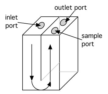
FIGURE 7.1. Representation of bed reactor with ports.
