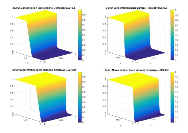
Figure 2: Field simulation: Behavior of the concentration of sulfur in the pore C(x, z, t) (left) and on the pore surface B(x, z, t) (right) at t = 316.8 days (top) and  $t = t_{\text{final}} = 524.3$  days (bottom).
